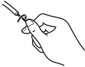
1: Strip the cover and twist the strands
